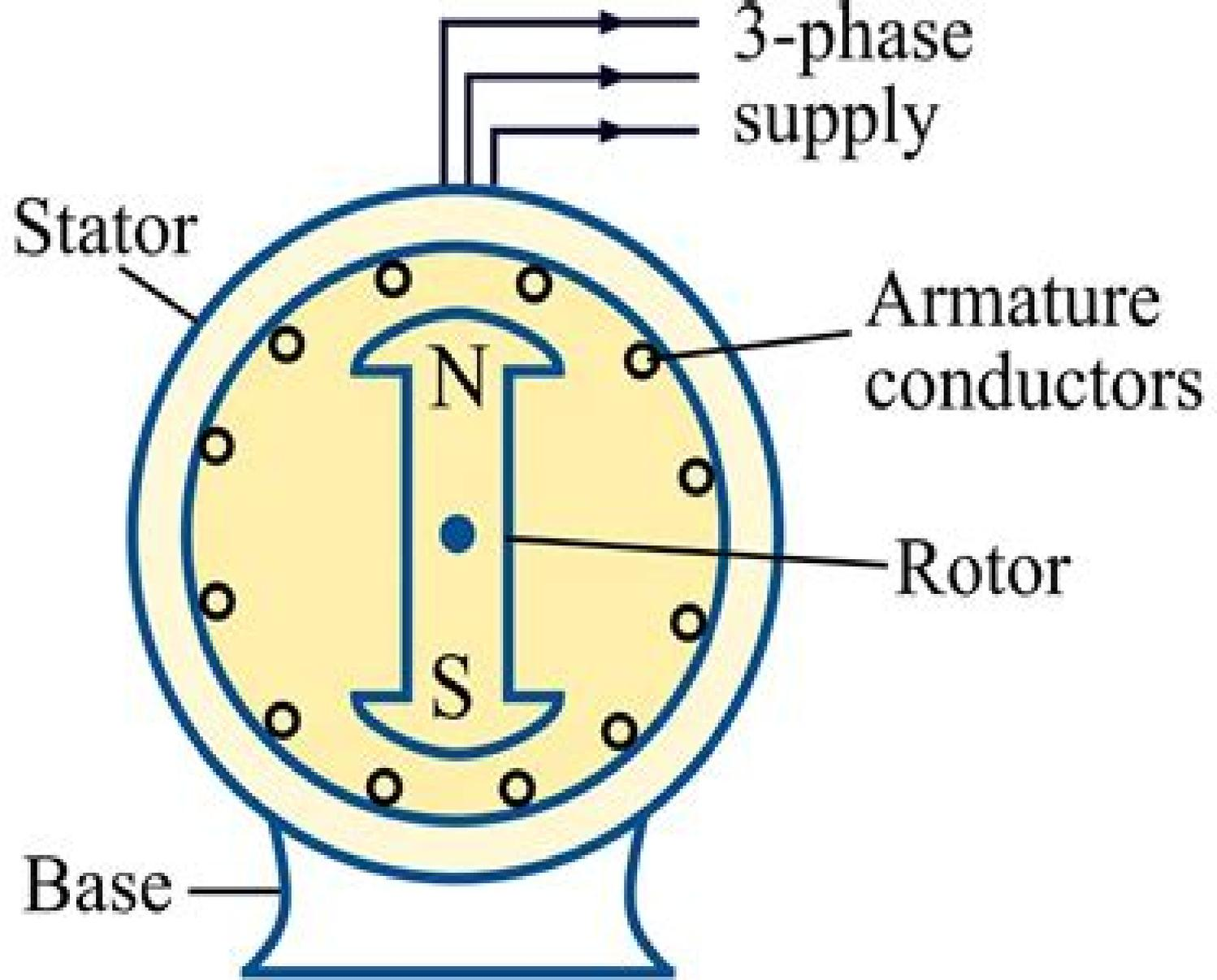
Figure 1 - Synchronous Generator
