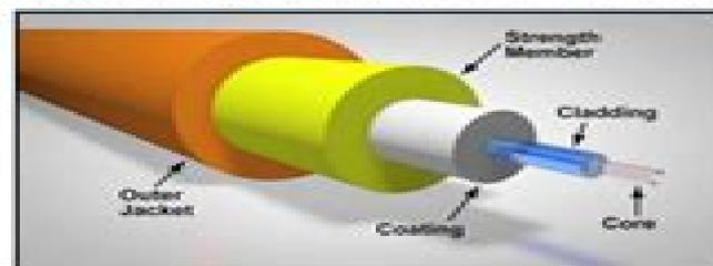
Fig. 5.1 Structure of optical fiber
