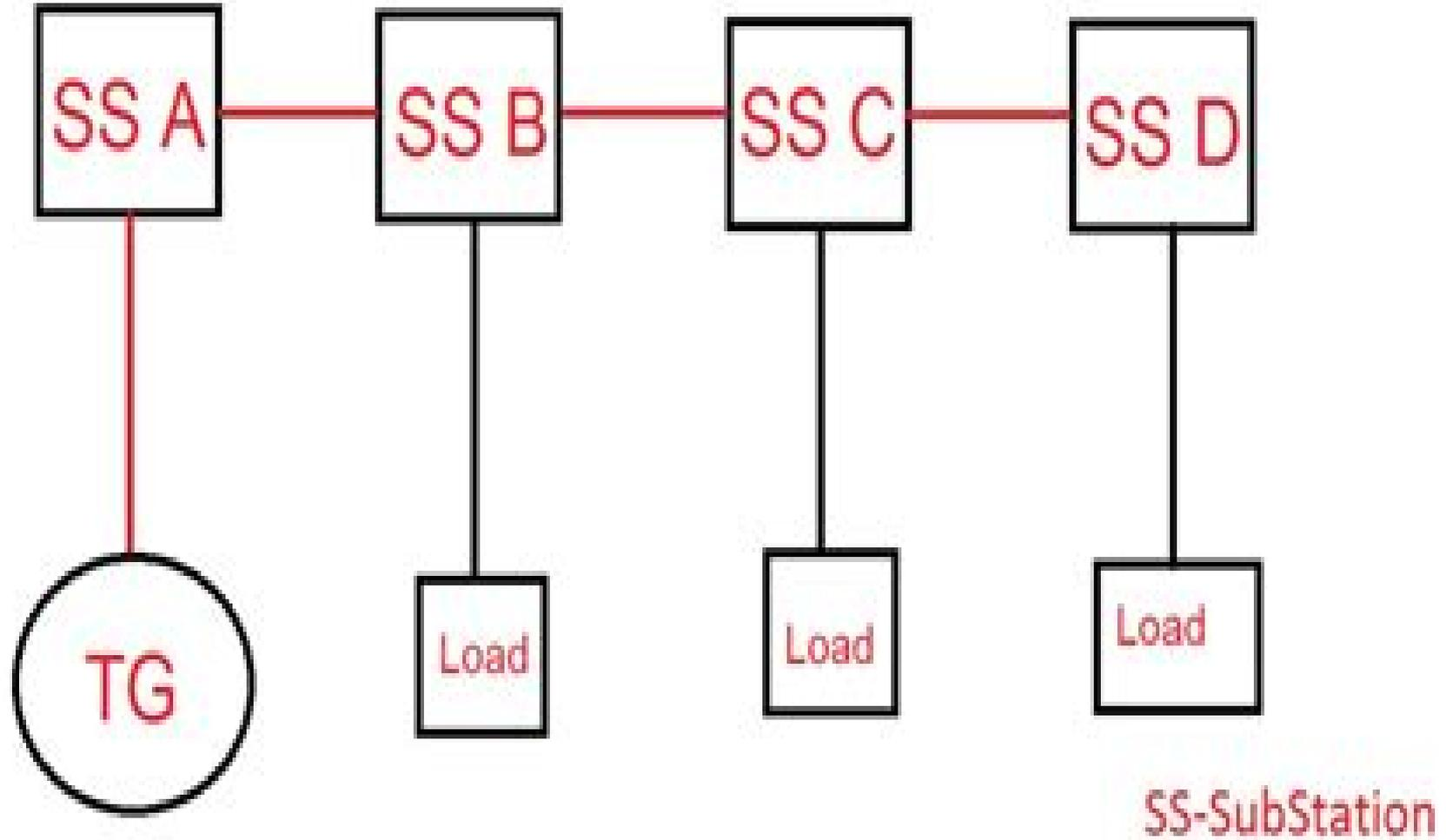
**Operating Time: Substation A > Substation B > substation C > Substation D.**
