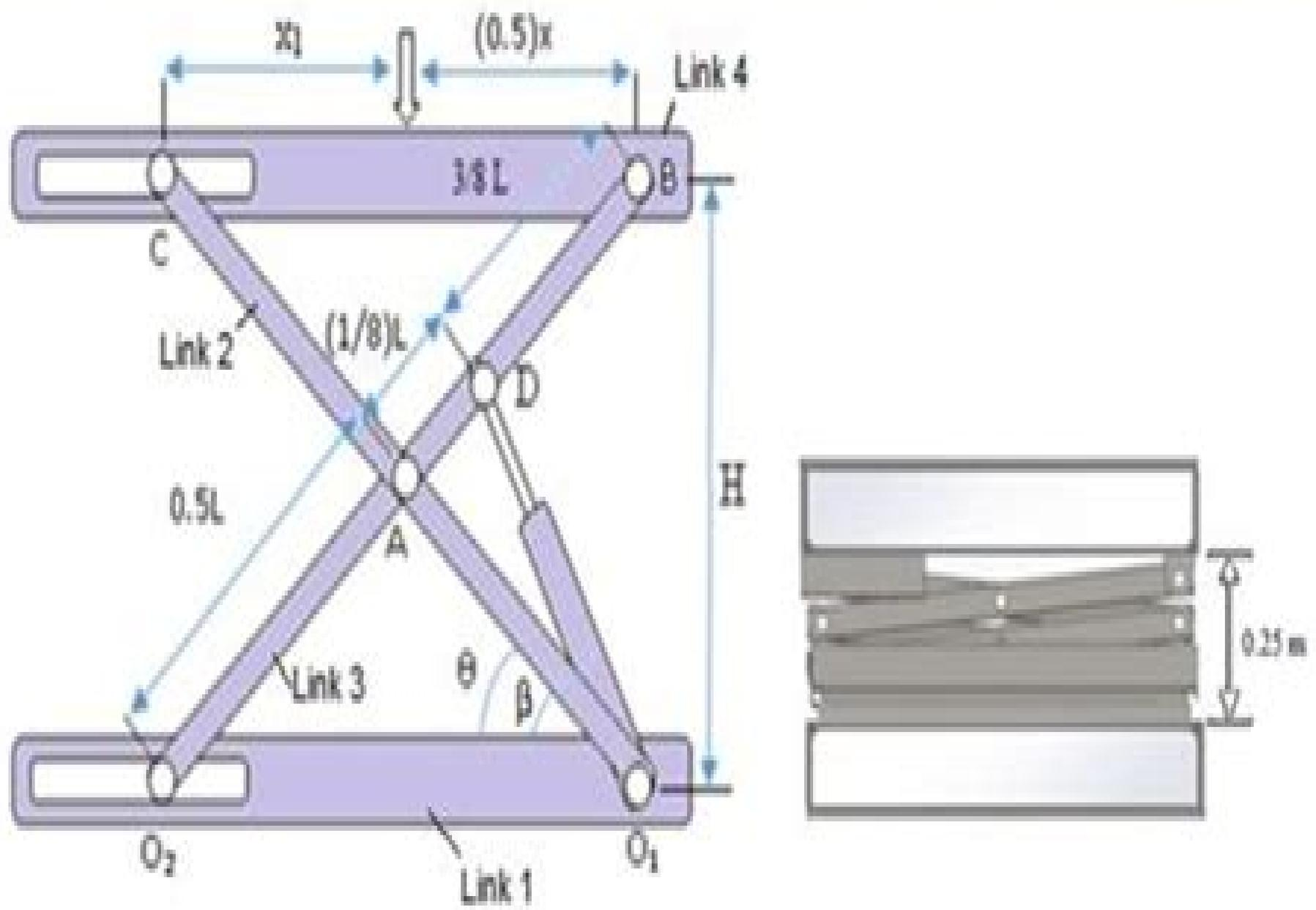
Figure 2: Geometry of Scissor Lift Mechanism [5]
